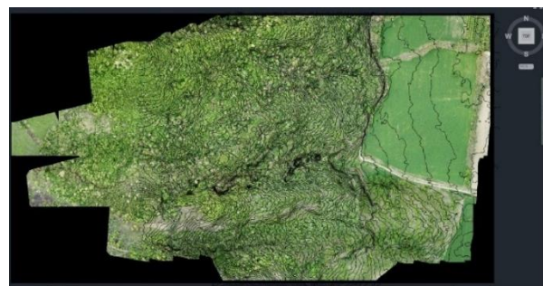
Fig.9. The resulted ortophoto plan and 3D DTM for the surveyed area Source: own processing.
